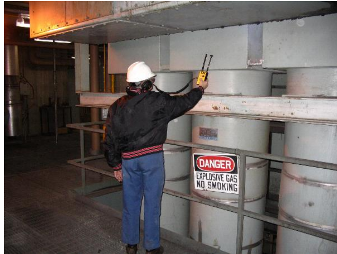
FIGURE 15: A hand held EMI detector is used to establish the location of a defect.
