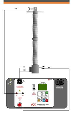
The Vanguard CVT-765 is a microprocessor-based, single phase, automatic, transformer turnsratio tester. This portable test unit is specifically designed to measure the turns-ratios of Capacitor Voltage Transformers (CVT's).
