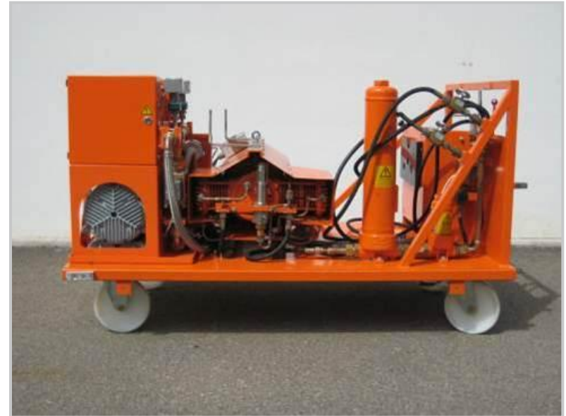
After modification with oil-free suction pump: gas recovery = 1 mbar
