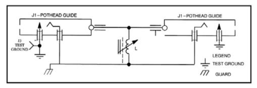
The simplified schematic diagram illustrates the Resonating Inductor. Note that the resonator electrically shunts the total specimen current; however, the measuring circuit is arranged to measure only the desired insulation current. The current taken by the Resonator is returned to its source without affecting these measurements.
