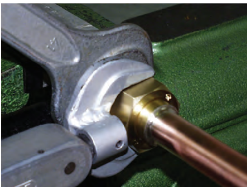
11. Tighten fast and strongly the clamping nut by counteracting force according to torque table
