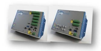
The Analytics unit also includes its own analog and digital I/O and extensive communication/hub capabilities and data back up; Doble PRIME Analytics will accept data from any standard condition monitoring device.
