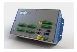
The Doble PRIME IDD measures the actual leakage current through the bushing tap, and measures the relative phase difference between the currents for each bushing in a set; voltage measurements will be recorded where available.
