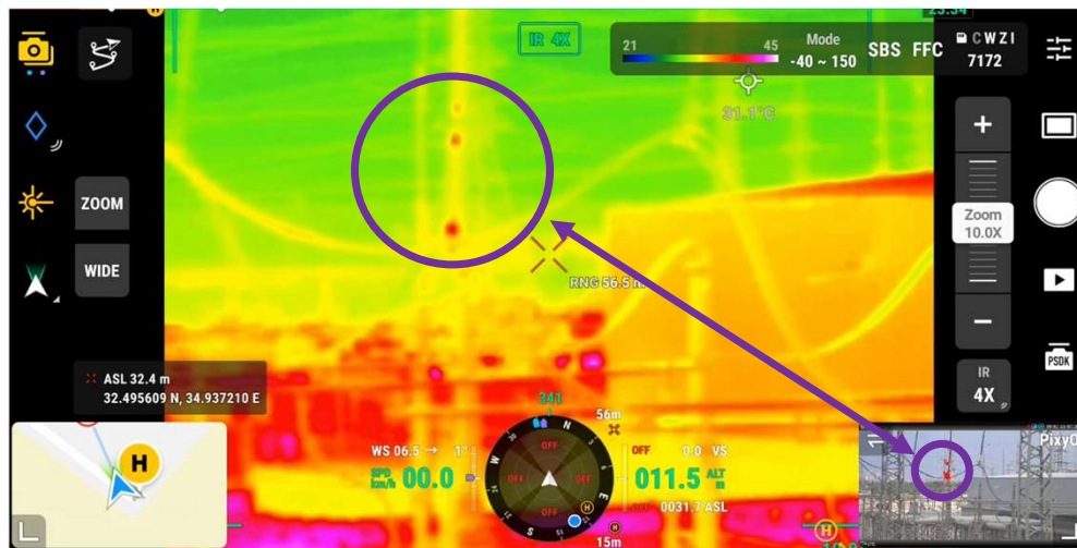
Corona PD Detection – Bushing
