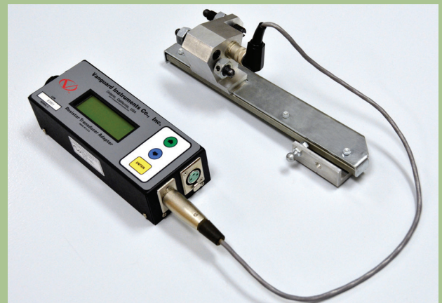
Connected to an ABB AHMB resistor-type transducer
