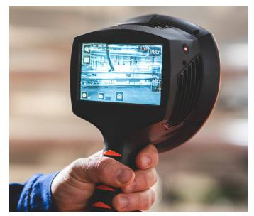
The NL Camera is a smart acoustic device for locating leaks in compressed air systems. The NL Camera automatically detects leaks by the sound that they emit, even in loud industrial environments. The device is lightweight and easy to use.
