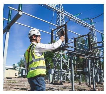
The NL Camera is an easy-to-use, stand-alone device for detecting and localizing partial discharges in medium and high voltage electrical systems during routine inspections. The NL Camera utilizes 124 microphones to find sounds emitted by partial discharges—even when they are completely inaudible to the human ear. Sound appears before components start to heat up, and the NL Camera enables detecting problems at an early stage.
