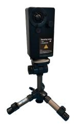
NL Sonic Tester is a reference sound source used to ensure the accuracy of the NL Camera.
